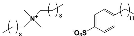
**Fig. 1. Didecyldimethylammonium dodecylbenzenesulfonate [DDA][ABS]**
