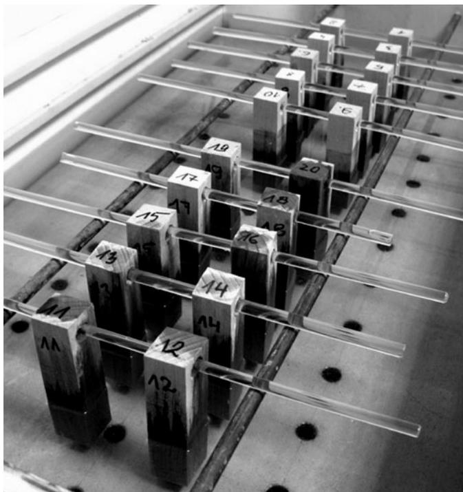
**Fig. 3. The samples during soaking in water (unprotected samples at the front)**
