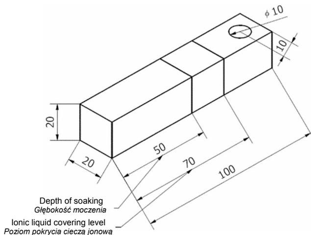
**Fig. 2. The sample used for swelling and water absorption tests**
