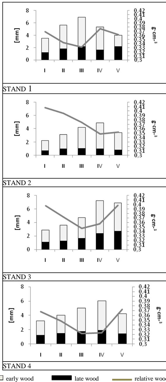
**Fig. 1. Variability of the wood properties under investigation along the radius of the trunk cross-section**
