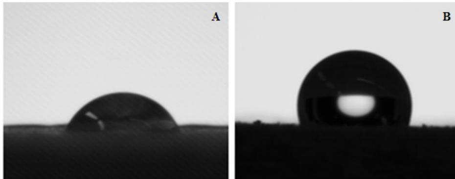
**Fig. 1. The image droplet water in wood surface. A: untreated wood (time = zero), B: treated wood with EKL (time = zero)**
