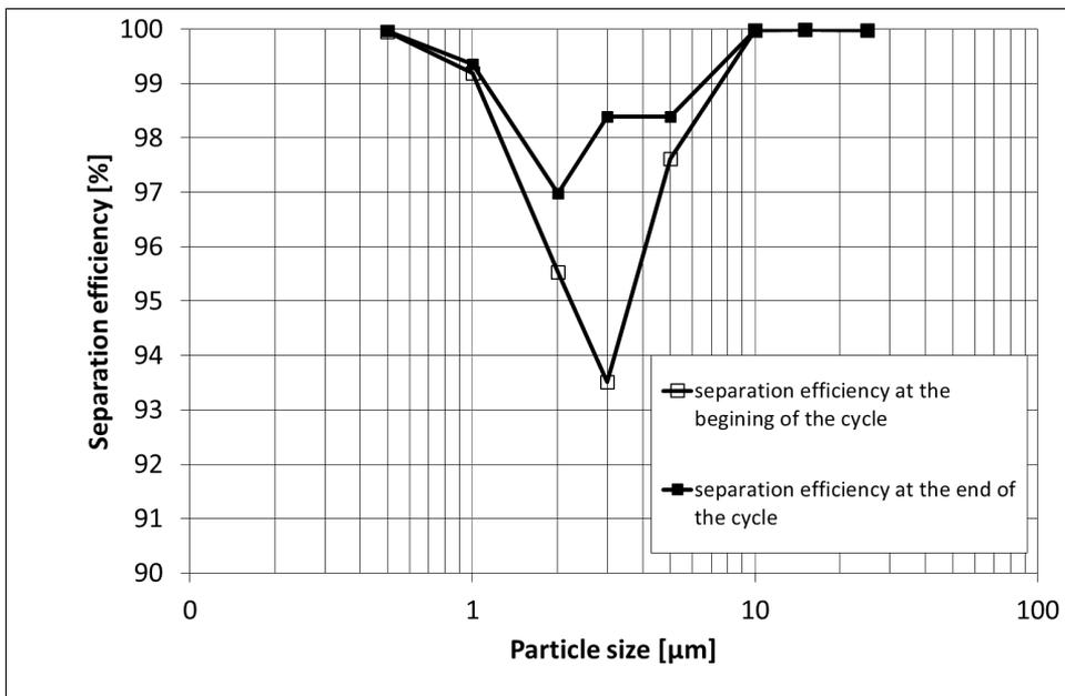
Fig. 4. Separation efficiency in the filtration cycle
