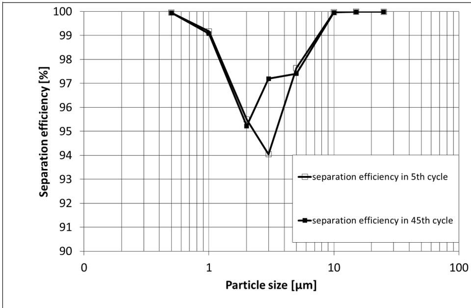
Fig. 3. Separation efficiency in the filtration process
