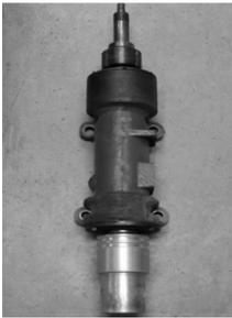
Fig. 3. Spindle with its bearing units
