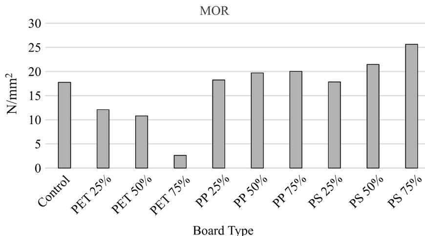
**Fig. 4. Bending strength values of tested boards**
