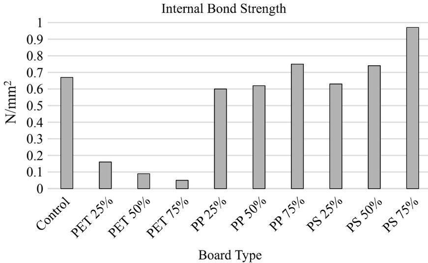
**Fig. 6. Internal bond strength values of tested boards**
