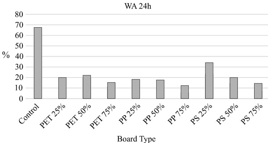
**Fig. 2. 24 h water absorption values of tested boards**
