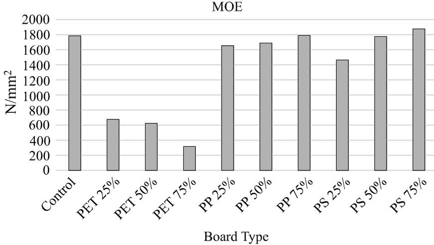
**Fig. 5. Modulus of elasticity values of tested boards**
