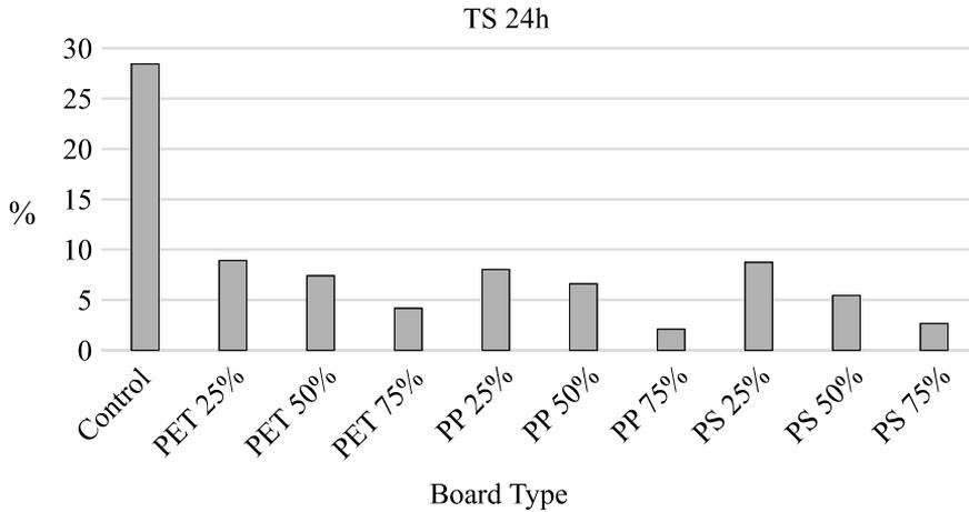
**Fig. 3. 24 h thickness swelling values of tested boards**
