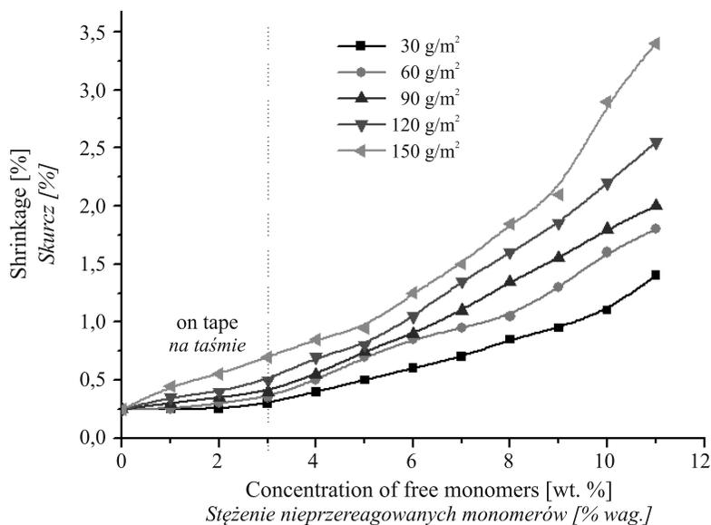
**Fig. 6. Shrinkage of self-adhesive tapes as a function of free monomers concentration**
