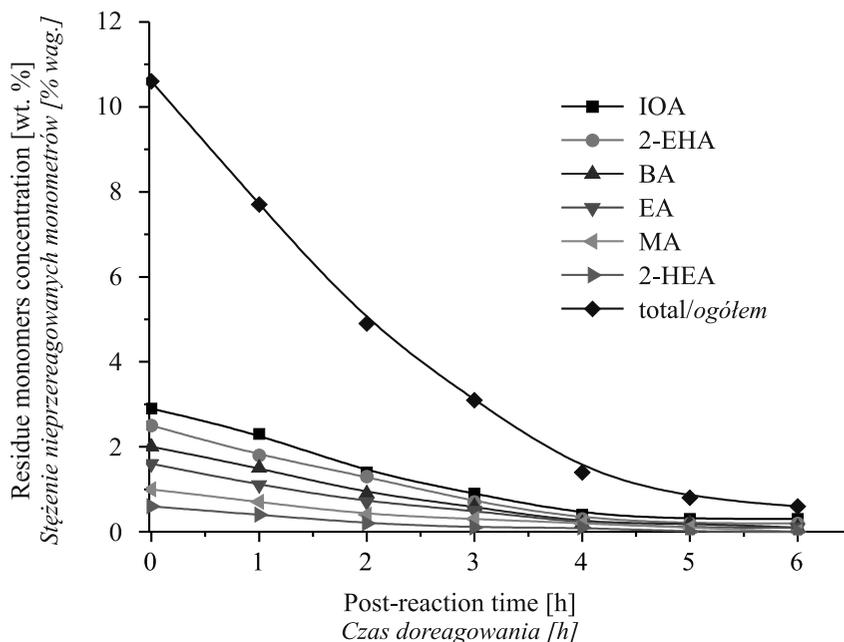
**Fig. 1. Concentration of residue monomers as a function of post-reaction time**
