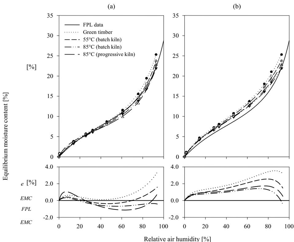
**Fig. 1. Sorption isotherms of green and dried Scots pine (*Pinus sylvestris* L.) at  $22\pm 1^\circ\text{C}$ . Upper plots – measured data and results of modeling using Hailwood-Horrobin ( $n = 2$ ) equation for (a) 1<sup>st</sup> adsorption, (b) 2<sup>nd</sup> desorption. Bottom plots – EMC differences between measured data and results of modeling**
