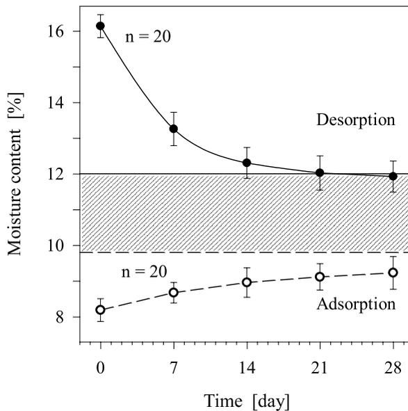
**Fig. 3.** Moisture content changes of 25 mm Scots pine timber dried at a temperature of 55°C (target MC = 10%) during storage at temperature of 20±2°C, RH = 55±5%, (striped area – sorption hysteresis, solid line – target MC for desorption phase, dashed line – target MC for adsorption phase)
