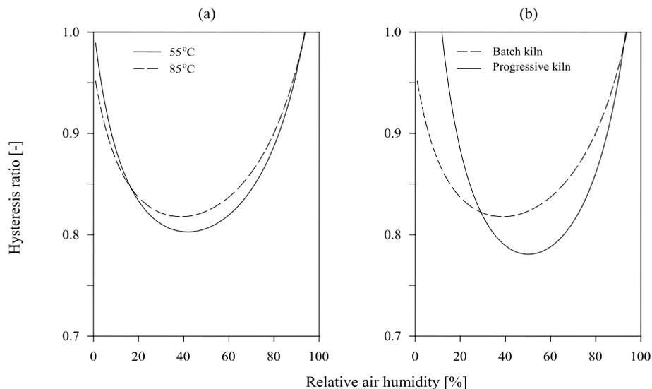
**Fig. 2.** Hysteresis ratio for *EMC* data obtained for 50 mm Scots pine timber (a) drying process in the batch kiln according to the mild schedule (temperature of  $55^\circ\text{C}$ ) and the severe schedule (temperature of  $85^\circ\text{C}$ ), (b) drying process in a batch kiln and a progressive kiln (temperature of  $85^\circ\text{C}$ )
