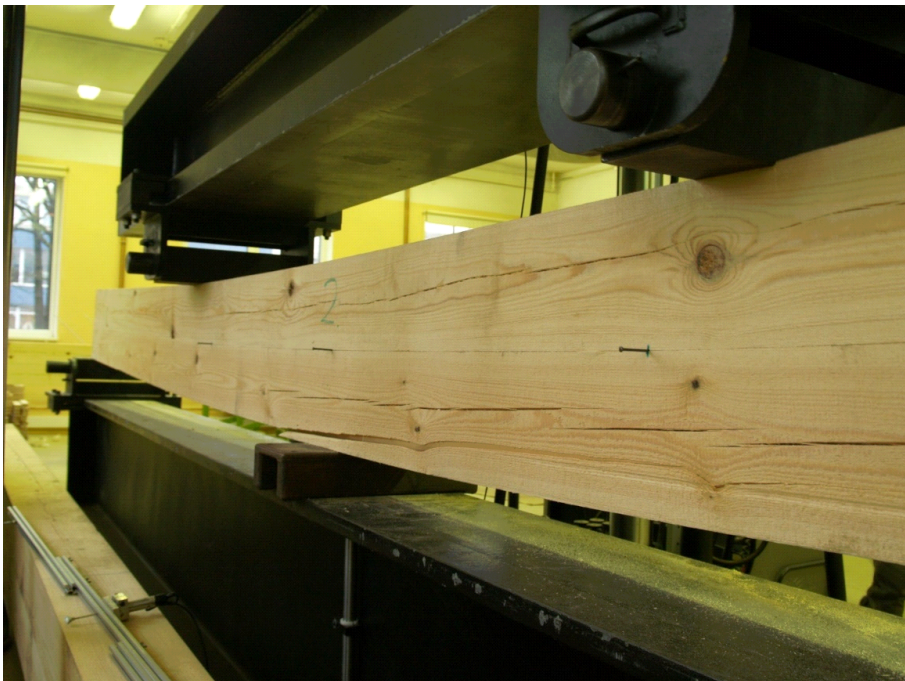
Fig. 3. Failure of experimental investigation specimen No.2
