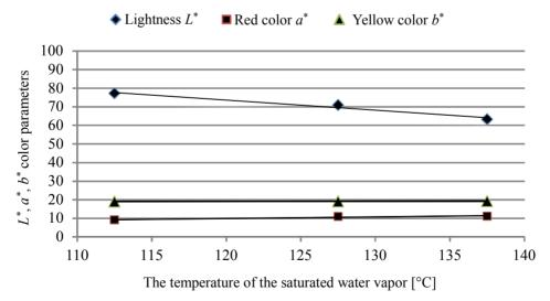
Fig. 3. Correlation of the decrease in lightness and the increase in red and yellow colour values of thermally treated maple wood, measured in the CIE- $L^*a^*b^*$  colour space, with the temperature of the saturated steam
