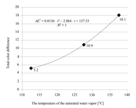
Fig. 4. Functional dependence of the total colour change of colour-modified maple wood, measured in the CIE- $L^*a^*b^*$  colour space, on the temperature of the saturated steam
