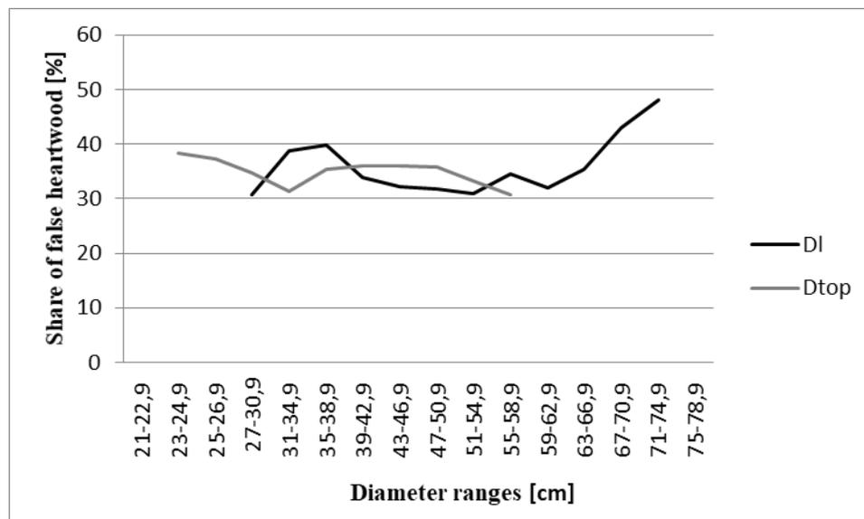
Fig. 1. The size of false heartwood depending on the butt-end diameter. ( $D_l$ )- lower log face; ( $D_{top}$ )- upper log face
