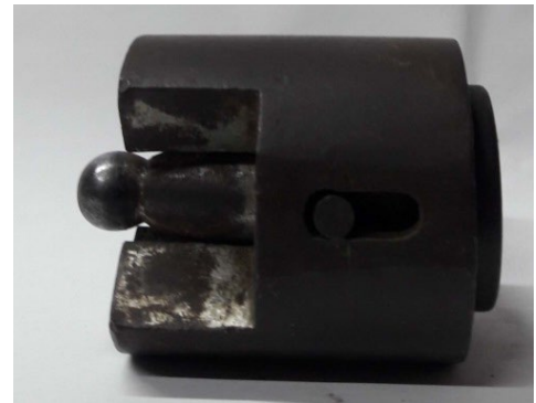
Fig. 5. Conducting experiment on static hardness of fir PCW
