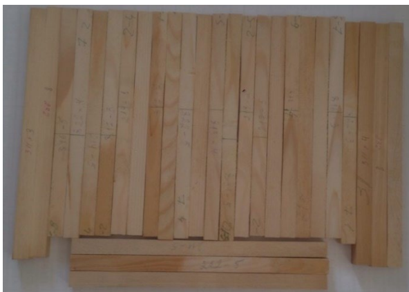
b) for static bending strength and modulus of elasticity in static bending tests
