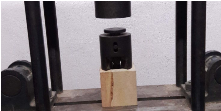
Fig. 5. Conducting experiment on static hardness of fir PCW
