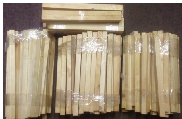
b) for static bending strength and modulus of elasticity in static bending tests
