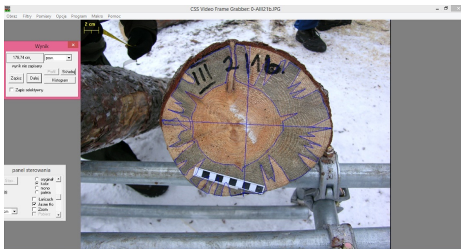
Fig. 2. Method of measuring the surface area of blue stain with the MultiScan program (photo taken during month 0) (photo by Wojciech Pasiowiec)
