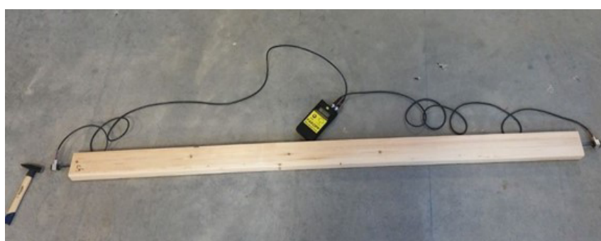
Fig. 4. Stress wave test setup to determine the dynamic MOE of the board
