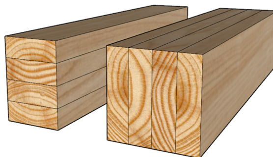
Fig. 1. Face-glued lumber manufactured in North America (left) and Europe (right)
