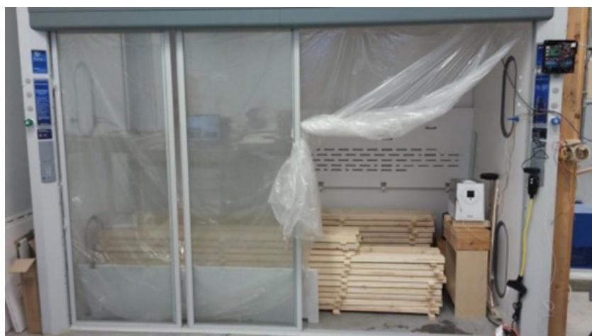
Fig. 3. Humidity chamber used to adjust the moisture content of specimens
