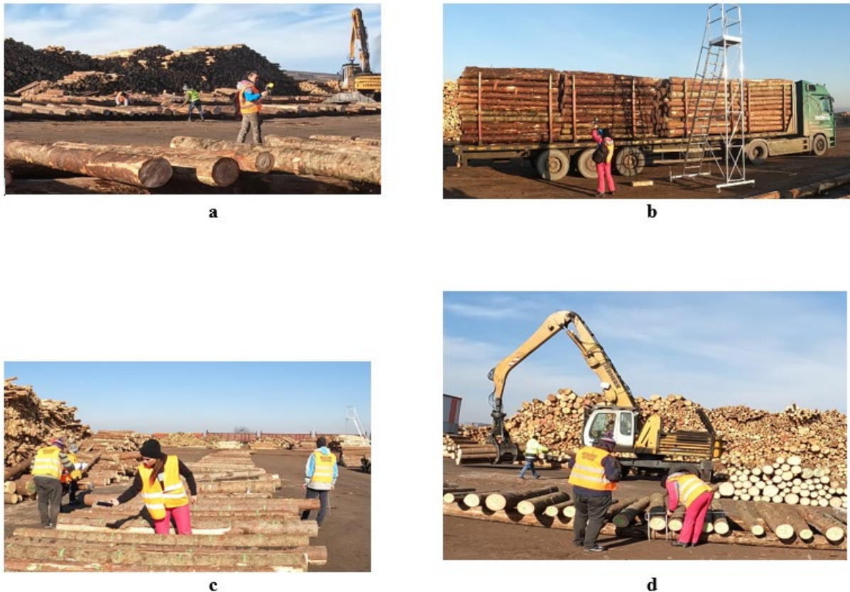
Fig. 1. Examples from measurement activities taken into study: a – scanning groups of logs at the ground by a professional LiDAR scanner (SLGZ), b – scanning piles of logs in the trucks by a professional LiDAR scanner (SLTZ), c – scanning individual logs at the ground by a smartphone (SLGP), d – measuring manually individual logs at the ground by a caliper and a tape (MM)
