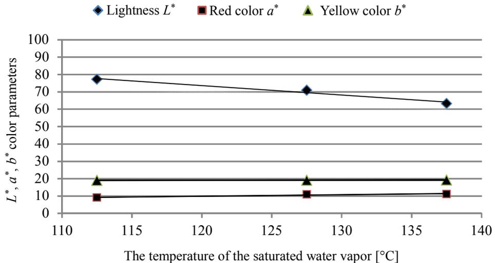
Fig. 3. Correlation of the decrease in lightness and the increase in red and yellow colour values of thermally treated maple wood, measured in the CIE- $L^*a^*b^*$  colour space, with the temperature of the saturated steam
